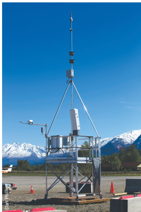
Left: Visual Weather Observation System (VWOS) platform after being installed at the Palmer airport site in early 2020.
