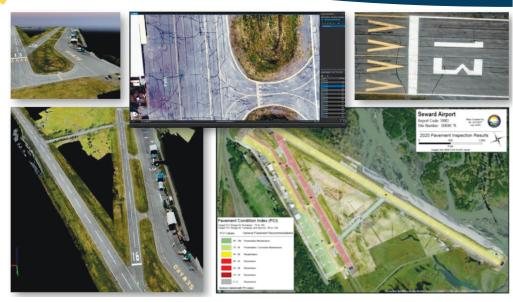
DOT&PF is utilizing drone technology combined with advanced computer analysis to pinpoint FAA compliance issues at the Seward airport.
