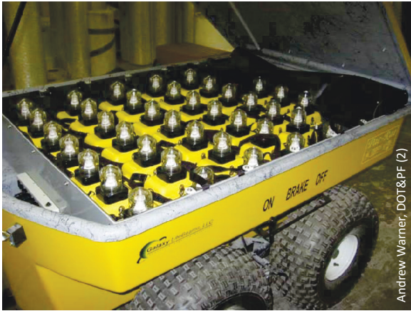
DOT&PF's emergency lighting trailers include 38 modular lights that can be pulled by an ATV or flown to rural airports. They can burn for up to 8 hours on a full battery charge.
