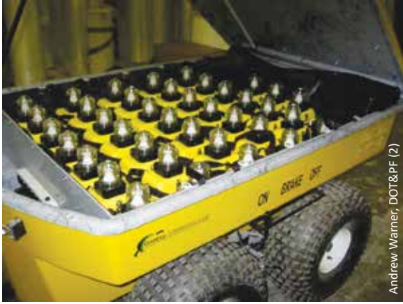
DOT&PF's emergency lighting trailers include 38 modular lights that can be pulled by an ATV or flown to rural airports. They can burn for up to 8 hours on a full battery charge.
