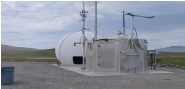
The Akutan Airport AWOS. This weather station was procured by the State of Alaska and is an example of a Non-Fed AWOS. Photo Courtesy of Jim Miller
