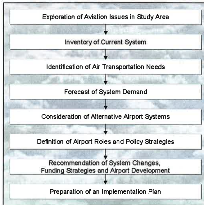
Figure 2: Airport System Planning Process
